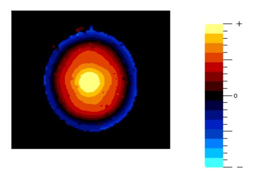
The image above is a laser vibrometer analysis, showing the expansion and contraction of the sphere. In contrast with conventional dynamic drive units, its reaction times are almost instantaneous. With reference to the graph below it is possible to see a comparative analysis of the impulse response.
