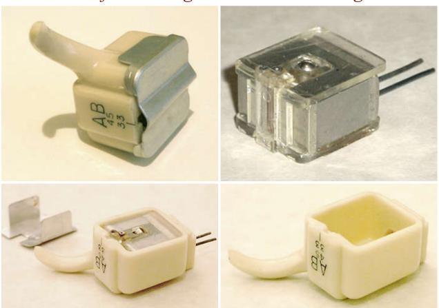
The early Ortofon mono moving coil cartridge was quite a heavy one. It showed already an important trait of the later Ortofon phono cartridges: the short aluminum cantilever.
