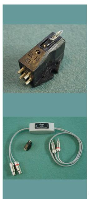
Ortofon SL 15 ELL is a further development of the Ortofon SL15 cartridge from around 1968 and had a beautiful step up transformer to match the impedance of the cartridge (2 Ohms) and the output impedance of 15 kOhm to connect perfectly well to the input impedance (load impedance) of 47 kOhm of the (pre-)amplifier. (These two images courtesy Don Sellers, USA).
