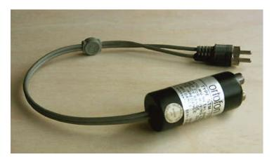
For the later SL-15E Ortofon developped a smaller and more affordable transformer, type STM 72 with a frequency range from 20 - 50.000 Hz., pick up impedance 2 Ohms, and load impedance 10 - 15 kOhm. The coils were double screened with mu-metal. This transformer could also be used with the MC20 and MC10.
