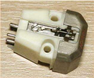
The cantilever is a long piece of metal that is fixed at one end with a bolt. On the other end figures a substantial stylus which asks for 4 gr. of playing weight. But since records in the mono era and in the first ten years of stereo were pressed from a harder and stronger vinyl, such weights were no problem. The Tannoy stylus could easily be exchanged for a new one or a special stylus for playing 78 RPM shellac records.
