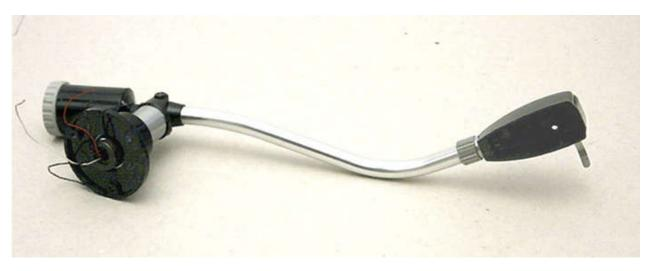
The simplest of Ortofon arms: short effective length, heavy counterweight to accommodate the headshell with cartridge and heavy transformer incorporated, rather soft plastic shell, no arm lift and no bias compensation.
