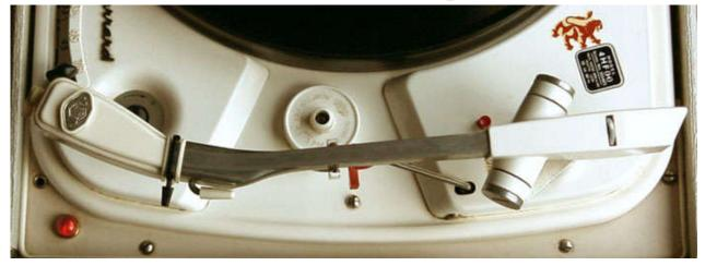
This is the Garrard TPA12 tonearm which adorns the 4HF and 5HF turntables and grammophones and the Type A record changer as well. Stylus pressure was adjusted by turning a wheel positioned at the rear end of the arm. In other versions adjustment was done by turning a bolt instead of a wheel.
